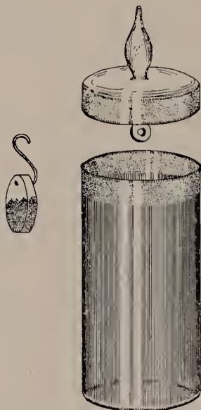
Fig. 19.—Author's weighing bottle for total solids in blood.
